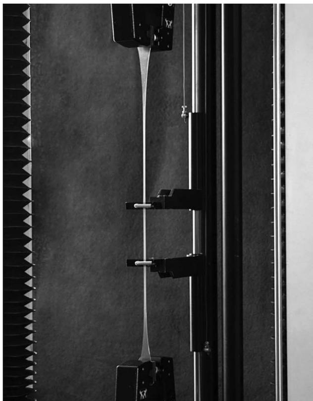
Fig. 1. Shell tension and elongation test.
