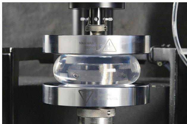
Fig. 2. Vertical compression test.
