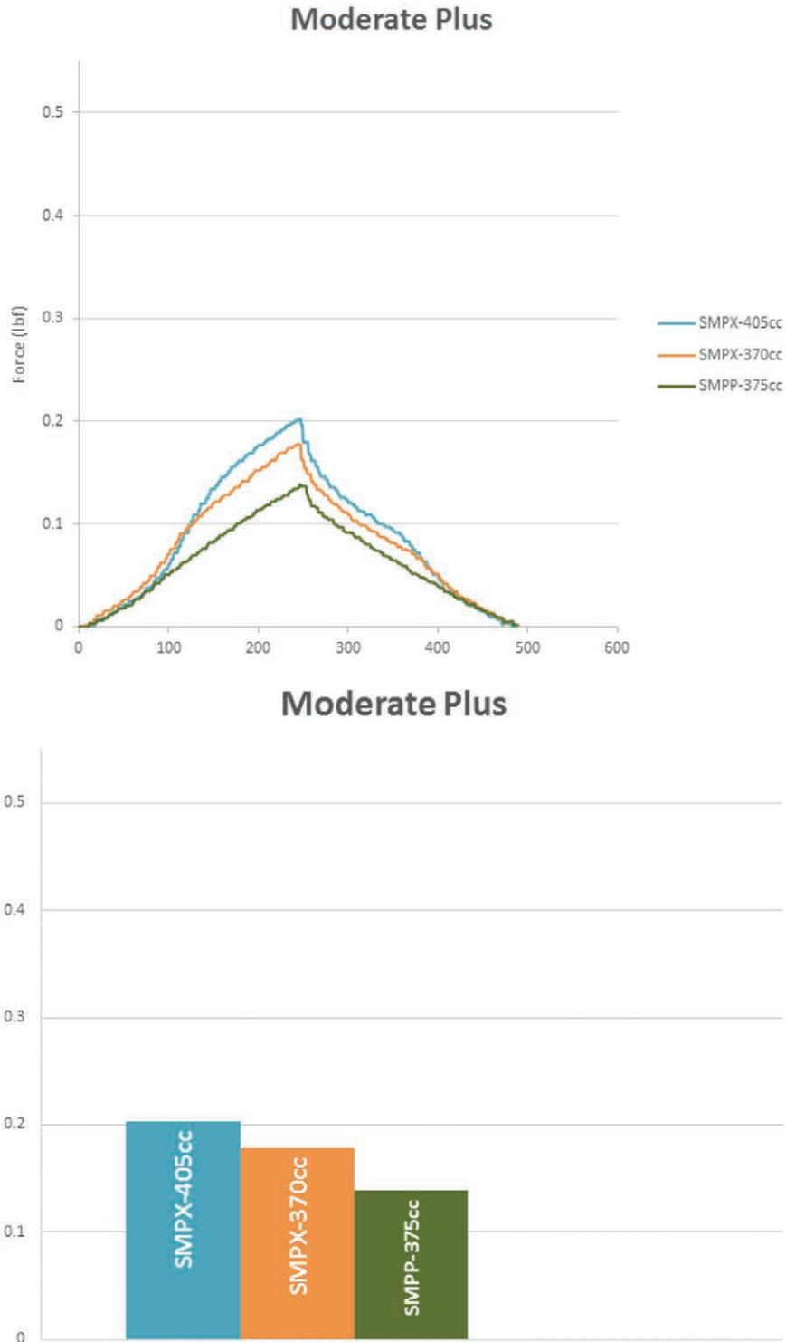
**Fig. 5.** Lateral compression test results comparing Mentor MemoryGel Xtra Moderate Plus Profile (SMPX) 405 cc and 370 cc to MemoryGel Moderate Plus Profile (SMPP) 375 cc demonstrating that MemoryGel Xtra Moderate Plus Profile implants are firmer than the current MemoryGel Moderate Plus implants.
