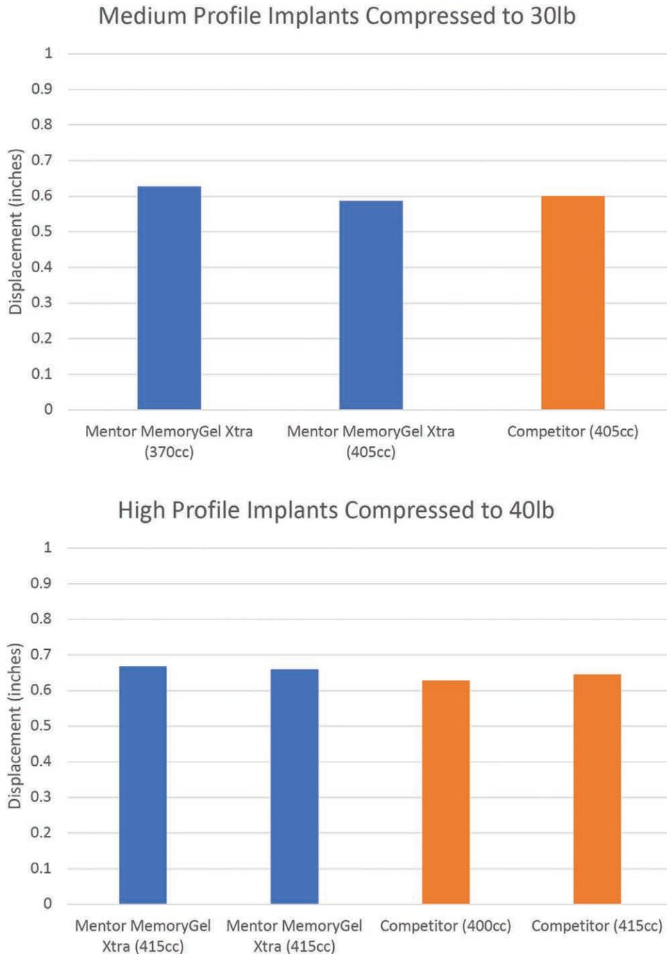
**Fig. 6.** Vertical compression benchtop testing (Strain-Energy testing) comparing High and Medium profile fully filled implants, compressed to (above) 30 lbs, and (below) 40 lbs, respectively.
