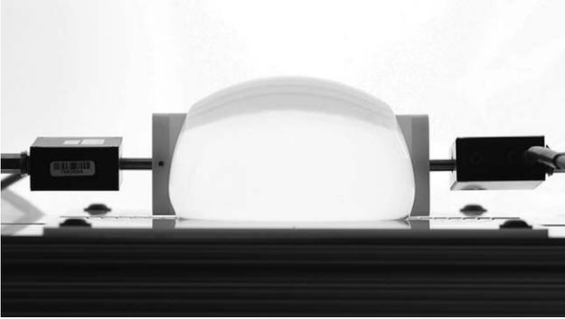
**Fig. 3.** Lateral compression test.
